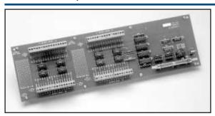
The MII-32 uses 4 consecutive addresses on the METRABUS. This allows up to 16 MII-32 boards (512 input points) to be connected to a single METRABUS driver board. The board is divided into four 8-bit ports. Reading a port returns the digital byte currently on the inputs.
